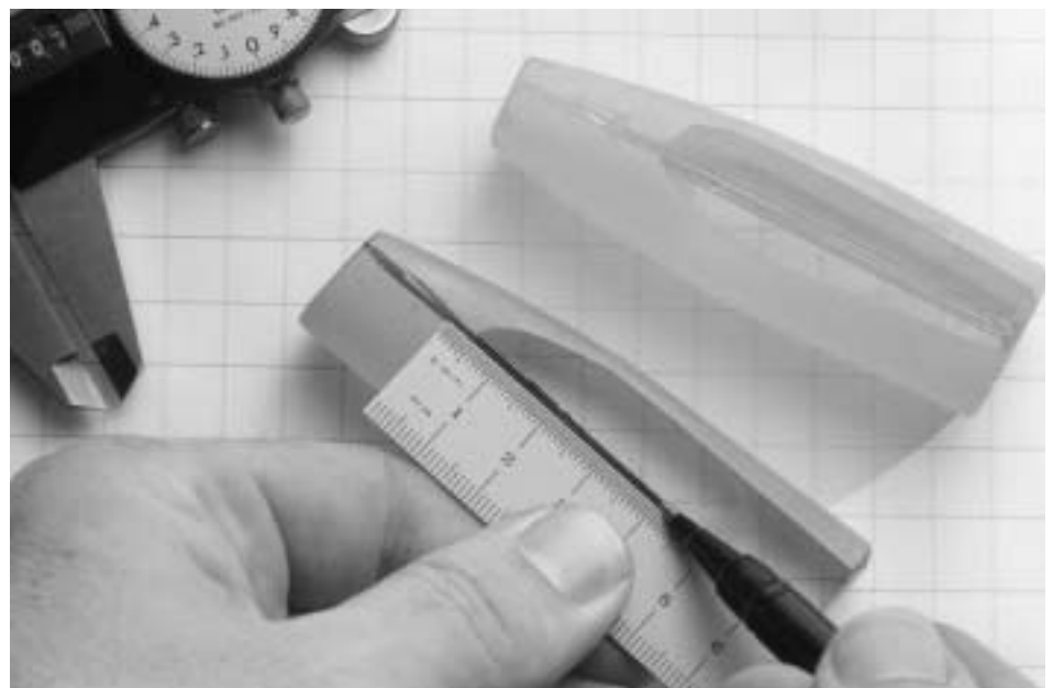
Preparing boule of Rutile for fabrication into prisms.
